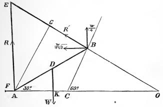
Let AC be the horizontal plane, CB the slope, and AB the ladder.
